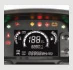
An advanced digital dash Standard on every Full-Size XUV. Monitors fuel level, speed (mph or km/h), RPM and coolant temperature. Plus, includes a clock, trip and lifetime odometer, 4WD indicator and hour meter.
