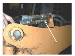
Arrow on fitting indicates flow through the hydraulic motor.
