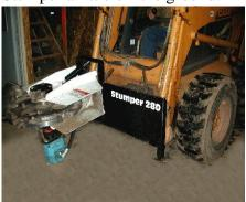
2. Secure latches on the skidsteer. Then lift Stumper so it is in the vertical position.
