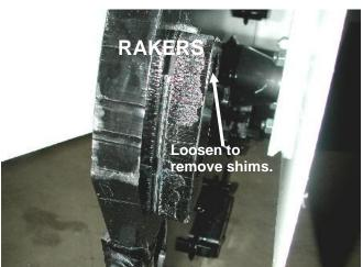
There is 1 Cutter Tooth with a shim located on the perimeter of the Cutter Wheel.
